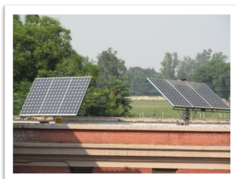
Fig 3b :Experimental setup with fixed stand(right) and dual axis tracking (left)
