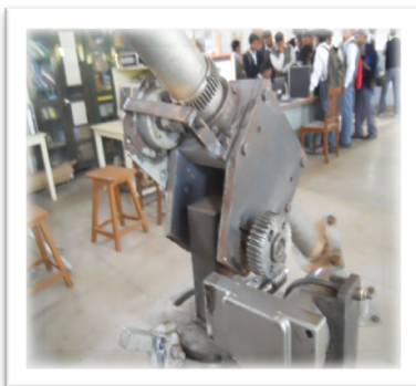
Fig 3a : Some of the prototype designs of 3 panel dual axis stands
